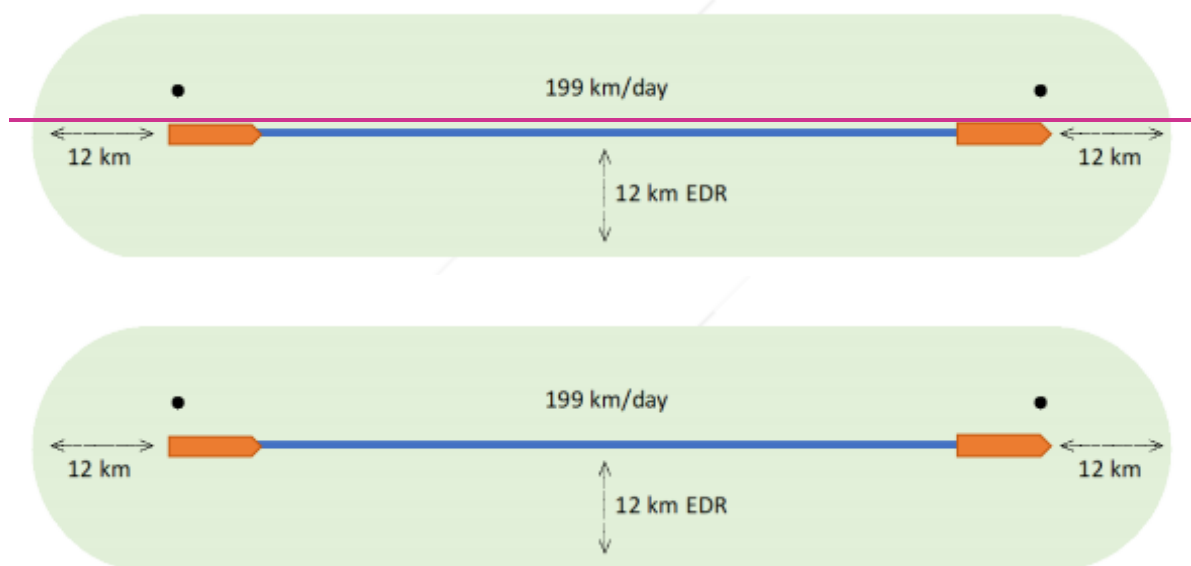
Graphic 11-1 Maximum worst-case theoretical area of impact over a single day from a seismic survey travelling at 4.5 knots using 12 km EDR (BEIS, 2020)
